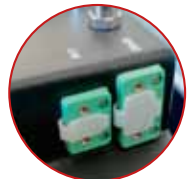
Display and CAN BUS connectors
